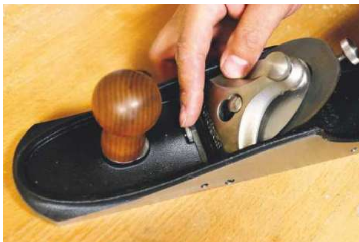
▲ This screw restricts the mouth to stop it clashing with the blade
